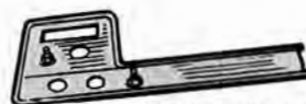
Regular style self-threading nuts are run down on molded studs of CB radio panel.
