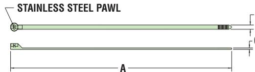
Material: Nylon 6/6 wire tie with a stainless steel locking pawl
