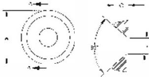
Available in natural or black nylon, these molded washers protect cabinets from scratching, cover misaligned holes, etc. May also be used as glides, bumpers, feet, and spacers.
