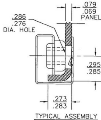
**G NUTS** combine the high strength of a multi-threaded nut and spring steel while eliminating the need for multiple tapped holes.
