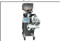
The only counters that utilize patented dual view scanners that provide the highest accuracy count possible. Out of tolerance parts are rejected prior to entering a package. An accurate high-speed counting system that detects and rejects parts one-third smaller or larger than a target part thereby separating the good parts from the bad. The processing unit is designed with a transparent front panel for visual inspection of gate movement and product flow.
